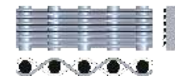
平纹席型网 PDW Plain Dutch Weave
