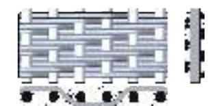
斜纹席型网 DTW Dutch Twilled Weave
