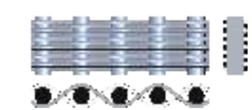
平纹席型网 PDW Plain Dutch Weave
