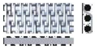
反向斜织席型网 TRD Twilled Reverse Dutch Weave
