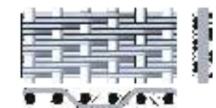
斜纹席型网 DTW Dutch Twilled Weave
