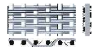
斜纹席型网 DTW Dutch Twilled Weave
