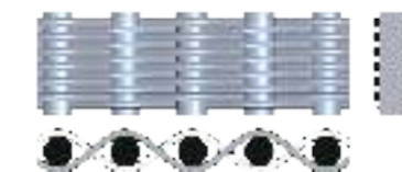
平纹席型网 PDW Plain Dutch Weave
