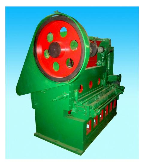
APM-25 type is a small expanded metal machine with function of punching and shearing, red 1.2 meters wide and the system ≤ 1.5 mm thick steel net, kind of expanded metal mesh is mainly used for mechanical, electrical, electronic, hardware, protective wait until the field. Punching board net of stainless steel, aluminum and other materials, and its use will become more widespread.
