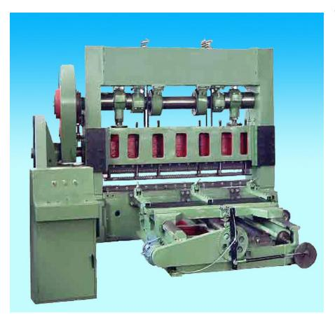
APM-100 type expanded metal machine is a heavy-duty punching machine, can be washed the system ≤ 4 mm thick steel net 2 meters wide, and the kind of expanded metal mesh is mainly used for shipbuilding, mining, machinery, construction, transportation, oil, urban construction, hardware, protective wait until the field.
