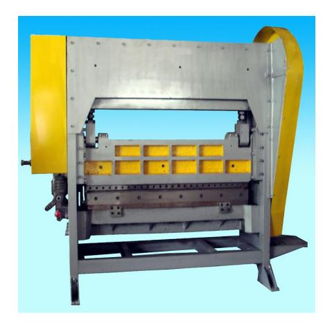
APM-16 type expanded metal machine is a small punching machine, red the system ≤ 1.2 mm thick steel net 1 meter wide, kind of expanded metal mesh is mainly used for mechanical, electrical, electronic, hardware, protective wait until the field. Can also be punched the board net of stainless steel, aluminum and other materials, and its use is very extensive.
