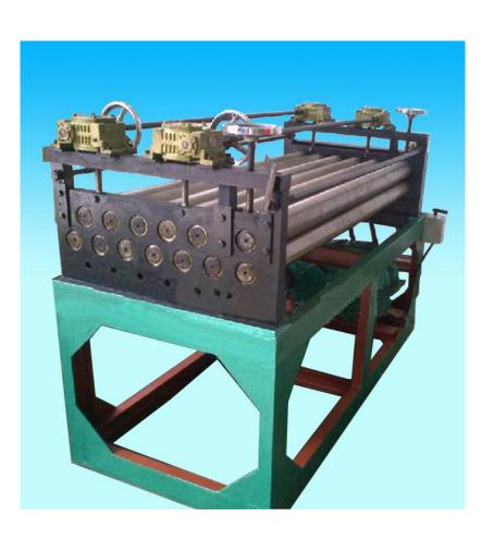
Sheet flatting machine: The expanded mesh will have a certain degree of bending out from the metal mesh machine, based on customer demand, we may be configured for the customers leveler the curvature leveling.
